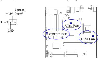
The two connectors, CPU\_FAN, SYS\_FAN are linked to the CPU fan, case fan, respectively. CHIP\_FAN can be used with North Bridge chip fan.
