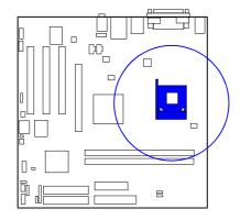
When you install your CPU on this mainboard, please use a power supply that designed and manufactured only for CPU use. Your CPU fansink combined with its retention module must be completely closed and firmly attached on the top of the processor.
