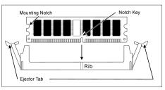
Do not force the DIMM module in with extra force as the DIMM module only fit in one direction.
