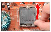
**3.** Use your right thumb on the bottom-right side of the load plate and lift it up to fully open position.
