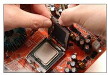
**6.** Use your left hand to hold the load plate, and use your right thumb to peel the cap off.
