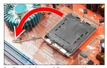
2. Rotate the lever to fully open position.
