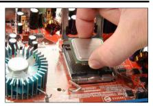
**4.** Use your right thumb and forefinger to grasp the CPU package. Be sure to grasp on the edge of the substrate, and face the Pin-1 indicator toward the bottom-left side. Aim at the socket and place the CPU package vertical down into the socket.
