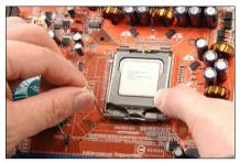
7. Lower the plate onto the CPU package. Engage the load lever while gently pressing down the load plate.
