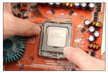
**8.** Secure the lever with the hook under retention tab.
