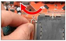
1. Place the board so as to let the lever hook of the socket is on your left side. Use your left thumb and forefinger to hold the lever hook, pull it away from the retention tab.
