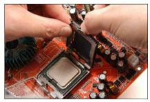
**6.** Use your left hand to hold the load plate, and use your right thumb to peel the cap off.
