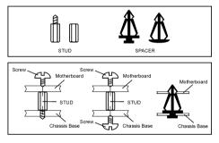
ATTENTION: To prevent shorting the PCB circuit, please REMOVE the metal studs or spacers if they are already fastened on the chassis base and are without mounting-holes on the motherboard to align with.
