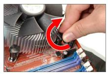
**11.** Rotate the fastener clock-wise to lock the heatsink and fan assembly into position.
