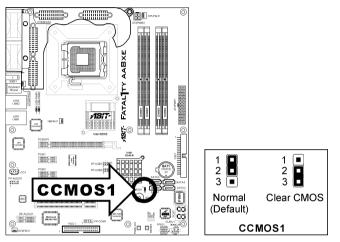
**WARNING:** Turn the power off first (including the +5V standby power) before clearing the CMOS memory. Failing to do so may cause your system to work abnormally or malfunction.
