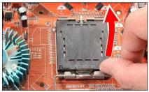
**3.** Use your right thumb on the bottom-right side of the load plate and lift it up to fully open position.
