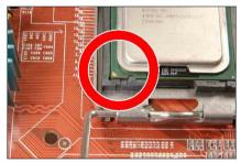
5. Visually inspect if the CPU is seated well into the socket. The alignment key must be located in the notch of package.
