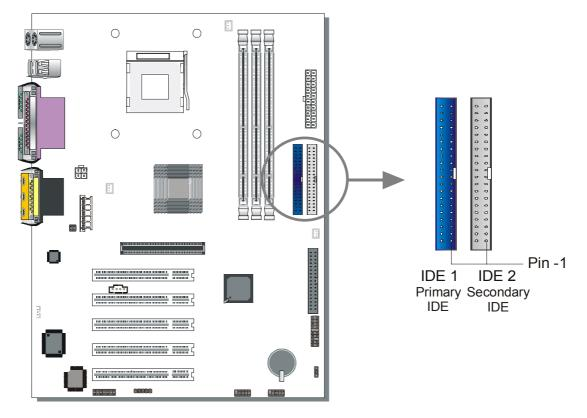
This Motherboard offers two primary and secondary IDE device connectors (IDE1, IDE2). It can support up to four high-speed Ultra DMA 33/66/100HDD or CD-ROM.
