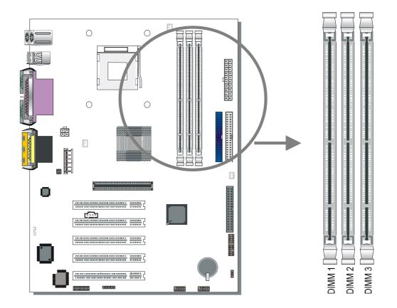
Your board comes with three DIMM sockets, Directly supports one SDR SDRAM channel, 64b wide, providing support max of 3 Double-Sided DIMMs with unbuffered PC133. *The largest memory capacity possible is 3GB.* On this motherboard, DRAM speed can be set independent from the CPU front side bus speed. Depending on the DRAM clock speed setting in the BIOS setup.
