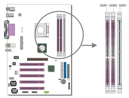
The P4VGA mainboard supports non ECC and non registered DDR and SDRAM modules.
