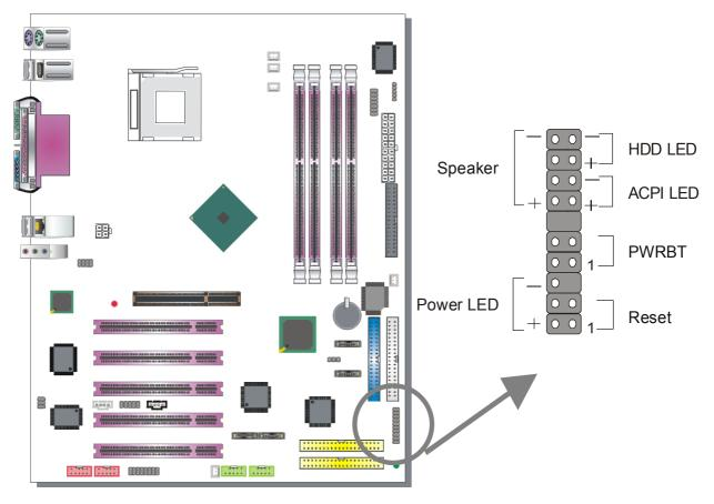
Plug the computer case's front panel devices to the corresponding headers on the Motherboard.
