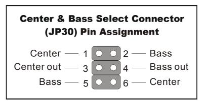
The 4 pin block jumper can be set to 1,2,3,4 or 3,4,5,6. The position this jumper block should be set to depends on your speakers. If during usage you find that your center and base channels are swapped set this jumper to the other position.
