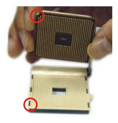
3. Seat the processor in the socket completely and without forcing.
