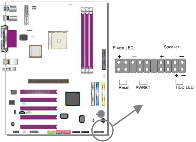
Plug the computer case's front panel devices to the corresponding headers on the Motherboard.
