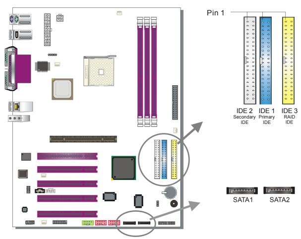
This Motherboard offers Three IDE connectors (IDE1, IDE2, IDE3) and 2 serial ATA ports. IDE1 and IDE2 can support up to four high-speed Ultra DMA 33/66/100/133 HDD or CD-ROM. IDE3 can support up to two DMA 33/66/100/133 HDD. CD-ROM is not supported on IDE3. SATA1 and SATA2 can support up to 2 ATA 150 SATA hard disks.
