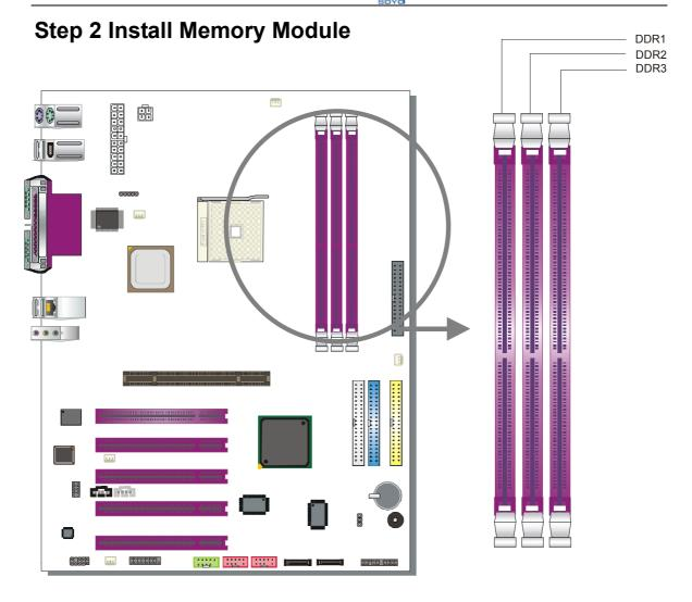
Your board comes with three DIMM sockets, providing support for up to 3GB of main memory. On this motherboard, DRAM speed can be set independent from the CPU FSB speed.
