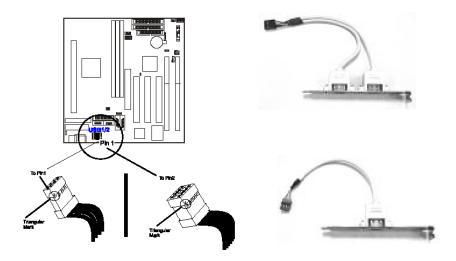
**External Front Panel Universal Serial Bus Connector: USB3**
