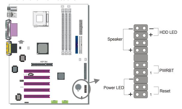
Plug the computer case's front panel devices to the corresponding headers on the Motherboard.
