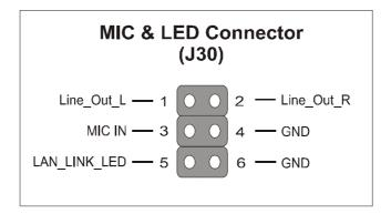
You can connect the Line-out /MIC in/LAN LED to the front panel of your PC case. (If this option is available in your PC case.)
