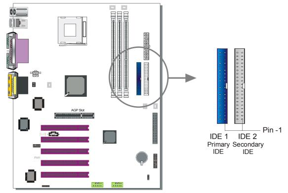
This Motherboard offers two primary and secondary IDE device connectors (IDE1, IDE2). It can support up to four high-speed Ultra DMA 33/66/100/133 HDD or CD-ROM.
