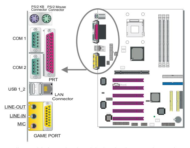
All external devices such as the PS/2 keyboard, PS/2 mouse, printer, modem, USB can be plugged directly onto the motherboard back panel.
