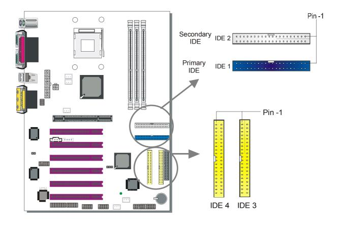
This motherboard offers two primary and two secondary IDE device connectors (IDE1, IDE2), can support up to four high-speed Ultra DMA 33/66/100/133 HDD or CD-ROM. IDE3, IDE4 can support up to four high-speed Ultra DMA 33/66/100/133 HDD. CD-ROM or other IDE peripherals is not supported on IDE3/4.
