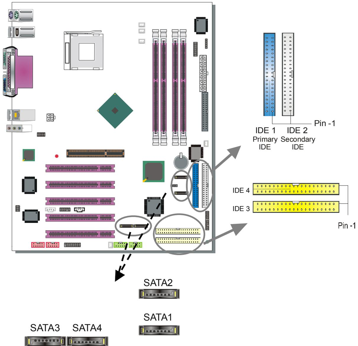
This Motherboard offers two primary (IDE1, IDE3) IDE device connectors, 2 secondary IDE device connectors (IDE2, IDE4) and 4 tertiary serial ATA ports. IDE1 and IDE2 can support up to four high-speed Ultra DMA 33/66/100 HDD or CD-ROM. IDE3 and IDE4 can support up to 4 high speed Ultra DMA 33/66/100/133 HDD. SATA1~4 can support up to 4 ATA 150 SATA hard disks.
