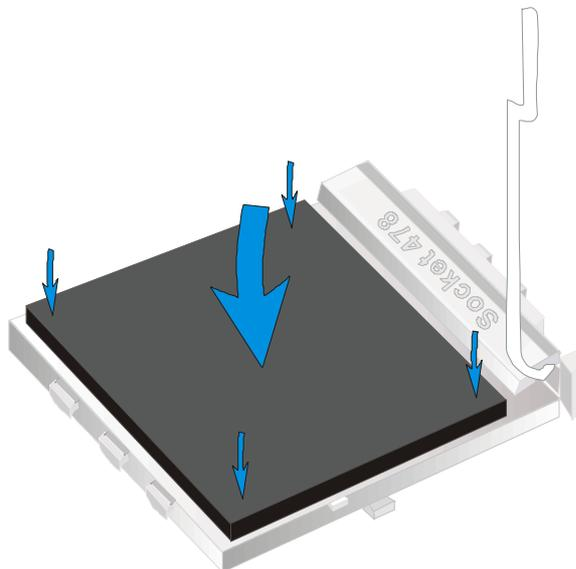
4. Then close the socket handle to secure the CPU in place.
