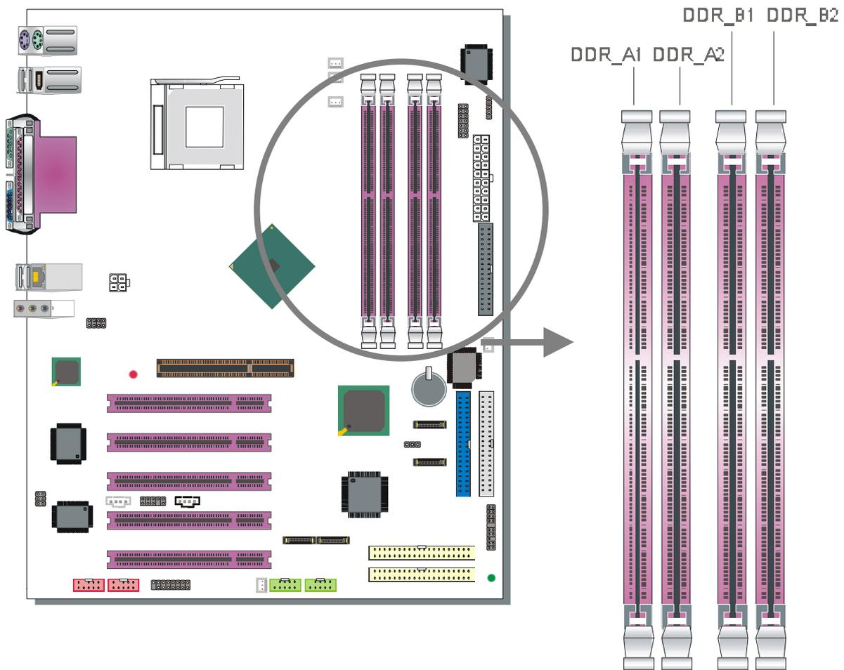
This motherboard supports two Dual Channels to your memory. Note that you can use normal DDR memory for Dual Channel to work. Also note that for Dual Channel to work 2 or 4 modules of equal size and specifications have to be installed.
