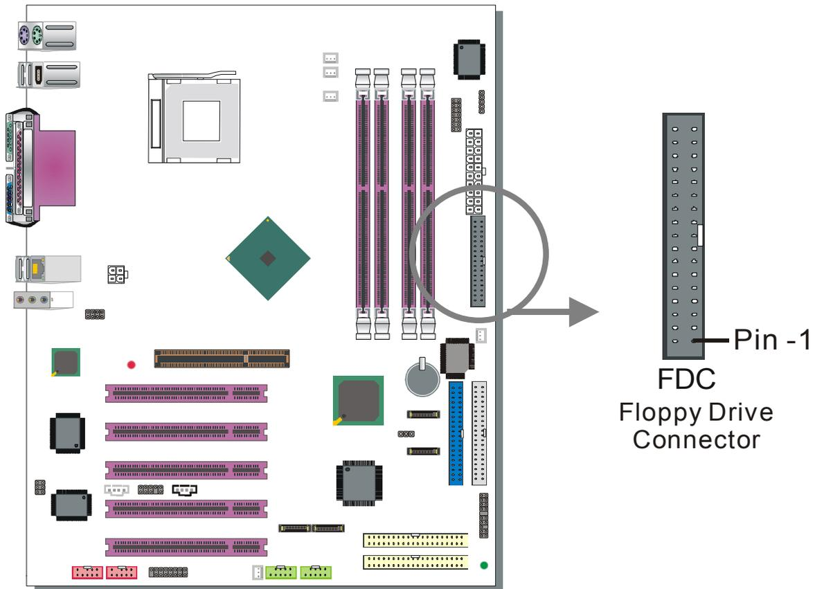
The system supports 5 possible floppy drive types: 720 KB, 1.2 MB, 1.44 MB, 2.88 MB. In addition, this Motherboard supports a 3-mode (720KB/1.2MB/1.44MB) floppy commonly used in Japan.
