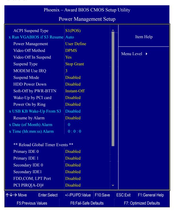
After you have completed the Power Management Setup, press [Esc] to return to the Main Menu.
