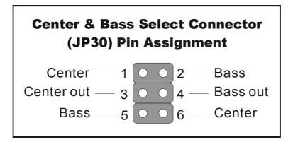
The 4 pin block jumper can be set to 1,2,3,4 or 3,4,5,6. The position this jumper block should be set to depends on your speakers. If during usage you find that your center and base channels are swapped set this jumper to the other position.
