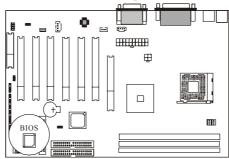
The BIOS IC is inserted in an IC socket, which means that it can be removed and exchanged for another IC if necessary.
