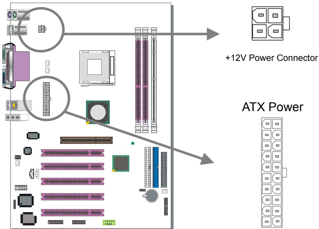
**Note1:** The presence of the +12 V power connector indicates that a power supply is ATX12V; the absence of the +12V power connector indicates that a supply is ATX.
