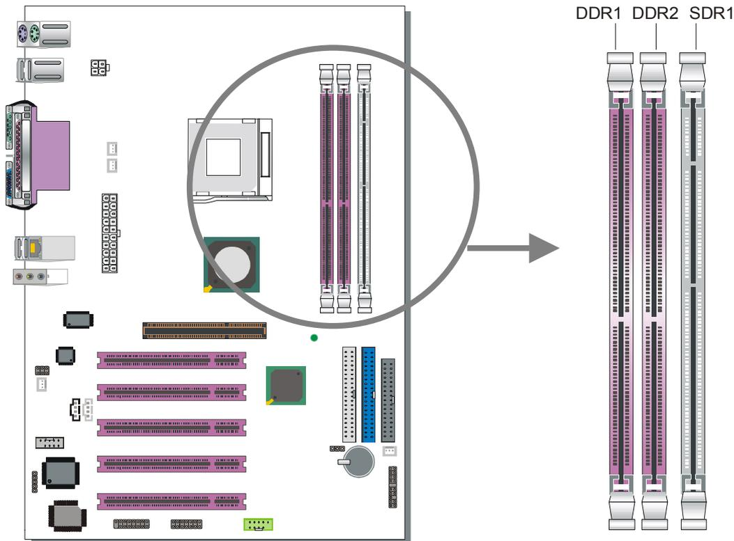
The P4VGA motherboard supports non ECC and non registered DDR and SDRAM modules.
