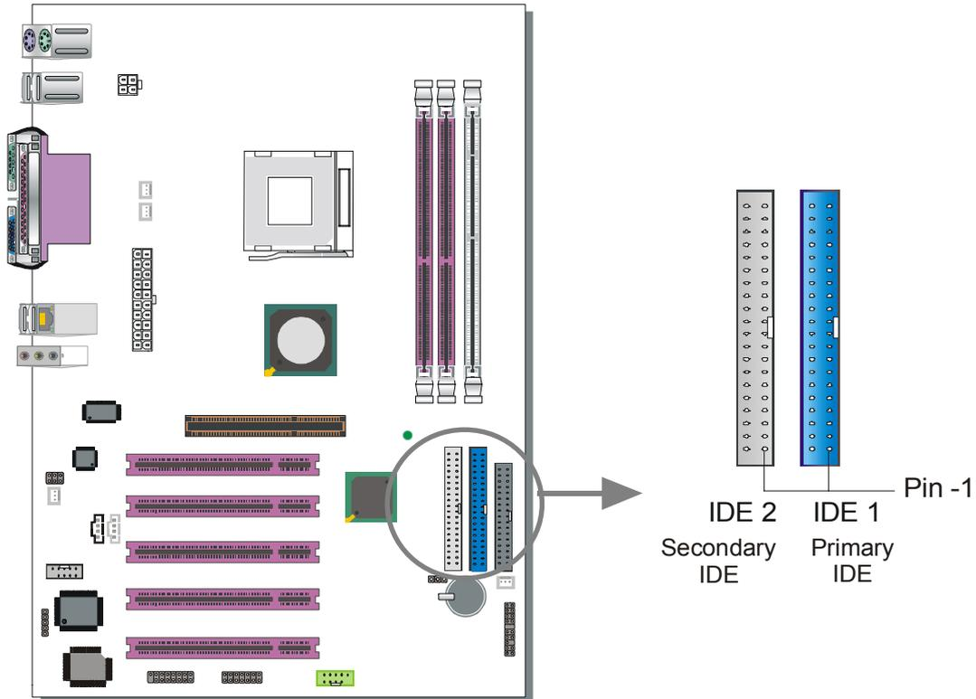
This Motherboard offers two primary and secondary IDE device connectors (IDE1, IDE2). It can support up to four high-speed Ultra DMA 33/66/100/133 HDD or CD-ROM.
