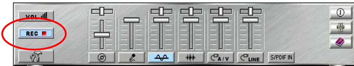
For each input signal, a control slider regulates the loudness whereas a horizontal slider the balance between the two channels. The select button can temporarily select input signal without changing slider positions. A button with a lit LED means it is available, and vice versa.
