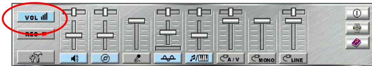
**Volume:** This is the master control over all outputs. The power of an output signal is determined by both of the volume slider and the slider for the individual output. To modify all the outputs, adjust the volume slider. To change individual output(s), adjust its(their) slider(s).
