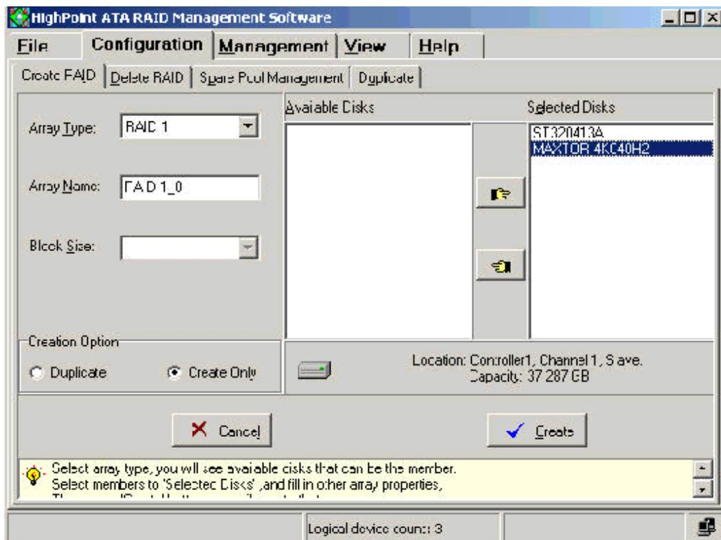
**Array Type:** Select the array type you want to create by RAID 0, RAID 1, JBOD and RAID 0/1 in this drop-down list box.
