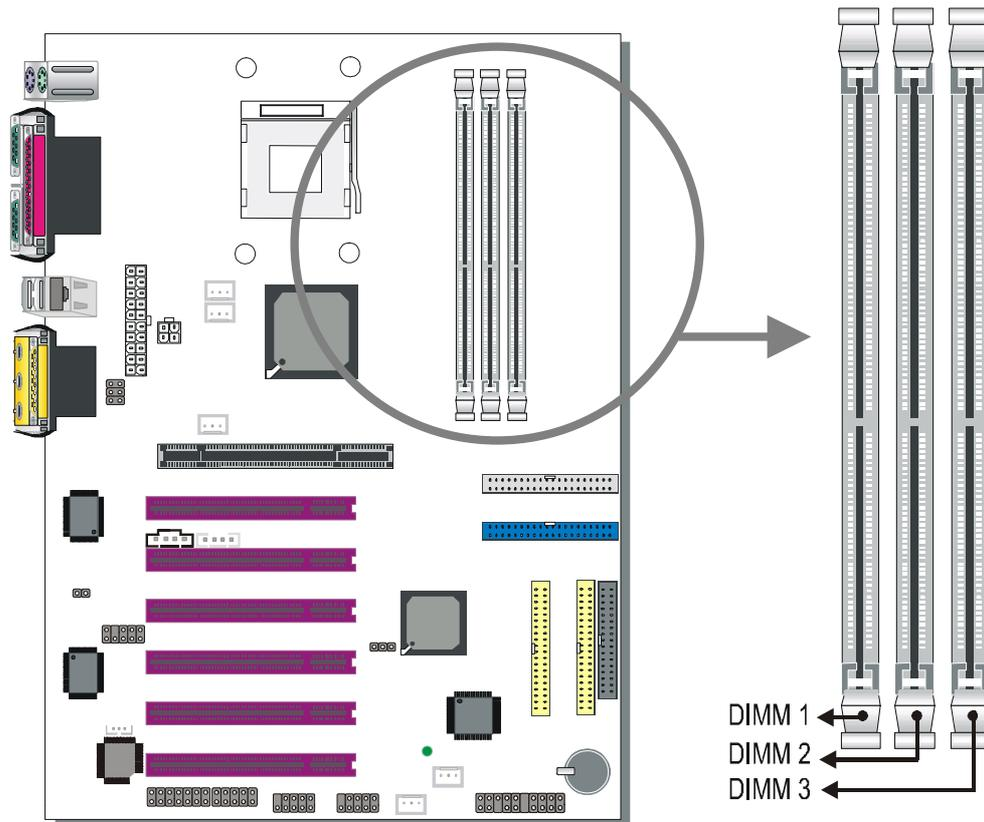
Your board comes with three DIMM sockets, providing support for up to 3GB of main memory using unbuffered DIMM modules from 64MB to 1GB. On this motherboard, DRAM speed can be set independent from the CPU front side bus speed. Depending on the DRAM clock speed setting in the BIOS setup, appropriate memory modules must be used. For 100MHz DRAM speed, use PC1600 memory; for 133MHz DRAM speed, use PC2100 memory; for 166MHz speed, use PC2700 memory.
