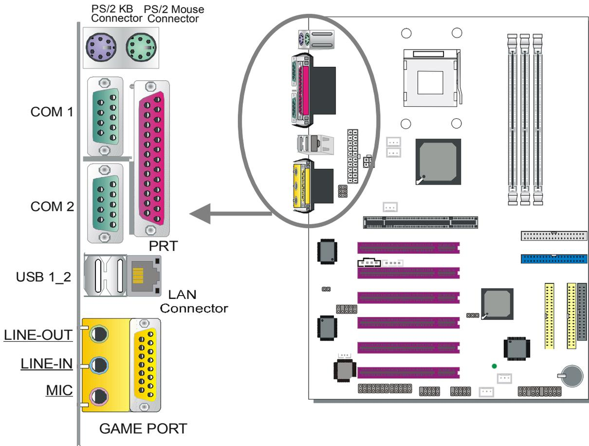
All external devices such as the PS/2 keyboard, PS/2 mouse, printer, modem, USB can be plugged directly onto the motherboard back panel.
