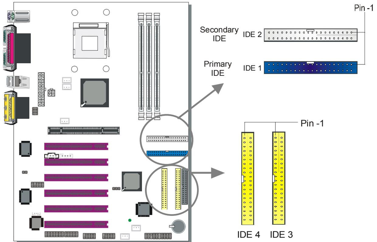
This motherboard offers two primary and two secondary IDE device connectors (IDE1, IDE2), can support up to four high-speed Ultra DMA 33/66/100/133 HDD or CD-ROM. IDE3, IDE4 can support up to four high-speed Ultra DMA 33/66/100/133 HDD. CD-ROM or other IDE peripherals is not supported on IDE3/4.
