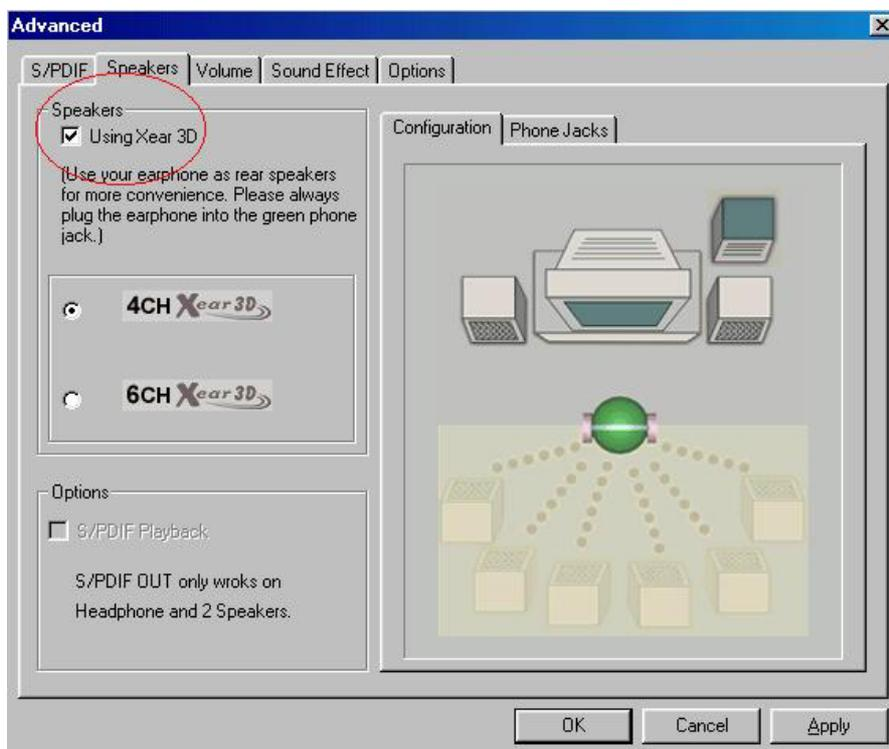
By clicking “Using XeaR” option, you can enter into XeaR Mode. **When choosing XeaR Mode, the driver will exchange the output channels of Front-Out and Rear-Out since the Rear-Out channels do not have earphone driving power. Therefore, users need to plug the front speakers into original Rear-Out phone jack and plug the XeaR earphone into Front-Out/Line-Out or Earphone jack as follows.**
