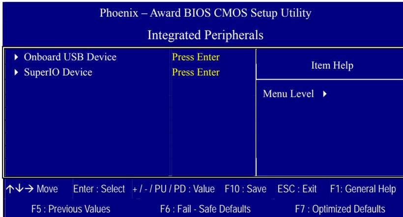
The following tables describe each field in the [INTEGRATED PERIPHERALS] Menu and provide instructions on how to configure the IDE controls, FDC controls, and the onboard serial and parallel ports.
