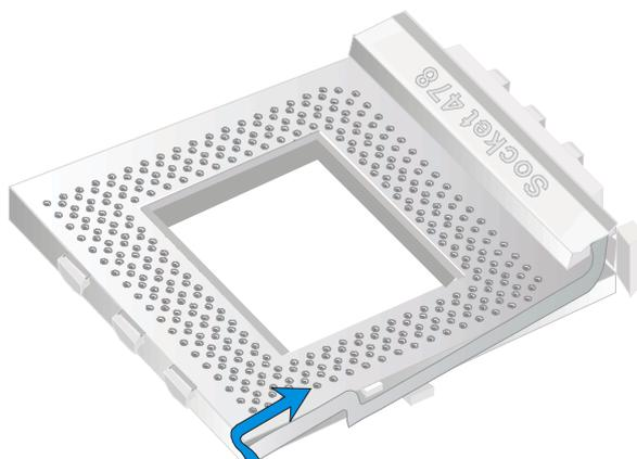
2. Align the blunt edge of the CPU with the matching pinhole distinctive edge on the socket.
