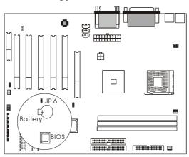
Normally JP6 will be in the 1-2 position, this will connect the battery to the southbridge of the chipset which contains the CMOS memory. If JP6 is temporarily set to 2-3 this will interrupt the battery electricity flow, and the CMOS memory will be erased, this will however only work if the power supply is not switched on. Now at the next reboot the BIOS will automatically load the CMOS default values.
