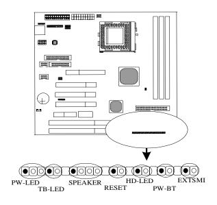
*PW-LED* is a 3-pin connector. It is used to connect to the LED on the case front panel. The LED shows the status of the power.
