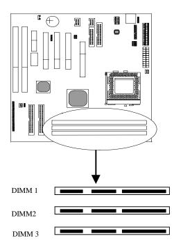
Insert the module as shown. Due to different number of pins on either side of the breaks, the module will only fit in the orientation as shown. There is no jumper setting for memory configuration.
