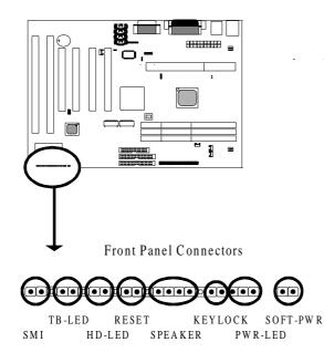
*SMI connector* is a 2-pin Berg strip, which is also called "green" or "sleep" connector. When SMI is turned from open to close and back to open, the system will enter sleep mode immediately. This function is to make sure power saving is working well. In PC system, it is used to connect to the push button SMI switch located on the case front panel (if there is). The system can be forced to power saving mode by pressing the SMI switch.
