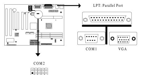
The onboard parallel port is a 25-pin female connector, marked as "LPT."
