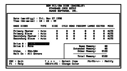
The "Standard CMOS Setup" allows user to configure system setting such as current date and time, type of hard disk drive installed in the system, floppy drive type, and the type of display monitor. Memory size is auto detected by the BIOS and displayed for your reference. When a field is highlighted (direction keys to move cursor and <Enter> key to select). The entries in the field will be changed by pressing <PageDown> or <PageUp> key or user can enter new data directly from the keyboard.
