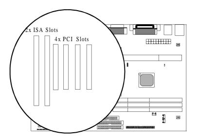
*There are* four standard PCI slots on board. 133MB/s data transfer rate on PCI bus can be compared to 33MB/s on EISA bus or 8MB/s on ISA bus. Synchronous operation CPU to PCI interface makes good graphic performance.
