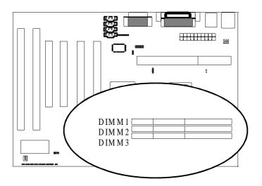
Insert the module as shown. Due to different number of pins on either side of the breaks, the module will only fit in the orientation as shown.
