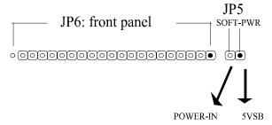
ATX soft-PWR switch connector is Soft-PWR with 2 pins.
