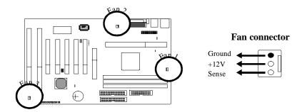
There are 3 fan connectors on this system board, and they are marked as "Fan 1," "Fan2," and "Fan3." Each fan connector has three pins.
