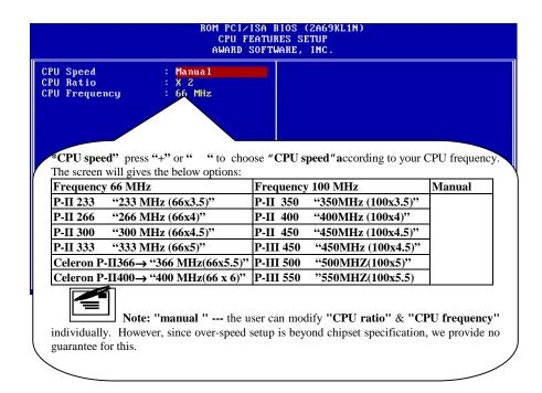
Since this is jumperless designed, there is no jumper setting to adjust CPU speed. The user only needs to set speed in BIOS. Please enter BIOS & find "CPU speed" item under "Chipset features setup" and set as above.
