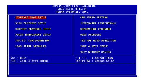
The menu displays all the major selection items and allow user to select any of shown item. The selection is made by moving cursor (press any direction key ) to the item and press **Enter>** key. An on-line help message is displayed at the bottom of the screen as cursor is moving to various items which provides user better understanding of each function. When a selection is made, the menu of selected item will appear. So the user can modify associated configuration parameters.
