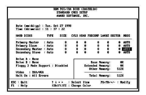
The "Standard CMOS Setup" allows user to configure system setting such as current date and time, type of hard disk drive installed in the system, floppy drive type, and the type of display monitor. Memory size is auto detected by the BIOS and displayed for your reference. When a field is highlighted (direction keys to move cursor and <Enter> key to select). The entries in the field will be changed by pressing <PageDown> or <PageUp> key or user can enter new data directly from the keyboard.
