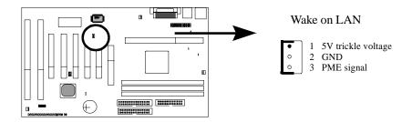
*Wake on LAN*, marked as "WOL," is a 3-pin connector. To support this feature, a network card is required for the system. More than that, a network management software must be installed too.
