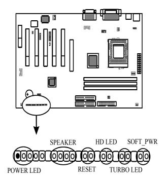
**POWER LED** is a 3-pin connector. It is used to connect the LED on the case front panel. The LED shows the status of the power.
