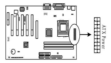
To support i815 chipset, we suggest that Pin 17 signal 5VSB on ATX Power supply should be able to offer at least 1A driving ability.
