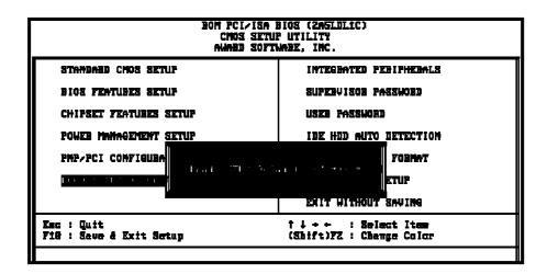
"Load Setup Default&bads optimized settings which are stored in the BIOS ROM. The auto-configured settings only affectBIOS Features Setup and Chipset Features Setup screens. There is no effect on the standard CMOS setup. To use this feature, highlight it on the main screen and press the Enter>key. A line will appear on screen asking if you want to load the setup default values. Press the and then press the Enter>key. The setup defaults will then load> Press if you don't want to
