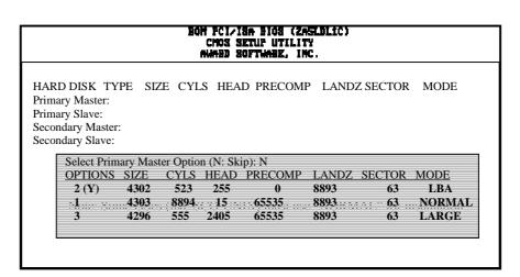
The "IDE HDD AUTO DETECTION" utility is a very useful tool especially when you do not know which kind of hard disk type you are using. You can use this utility to detect the correctionsk type installed in the system automatically or you can set hard disk type to auto in the standard CMOS setup. You don't need the "IDE HDD Aauto Detection tility. The BIOS will auto-detect the hard disk size and model on display during post.
