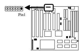
IR uses the same I/O port as COM2. There is no hardware jumper setting for I.R./COM2 on this main both buter needs to set proper BIOS (refer to page 32) setup for "HP SIR," "ASKIR," or "Disabled" (default) under "IR Address Selection" of intergrated Periphærædæding to the following table.
