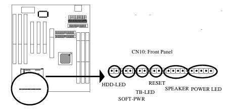
*Marked "HDD-LED*," Hard Disk activity LED connector is a 2-pin keyed Berg strip. It is used to connect to front panel Hard Disk LED.
