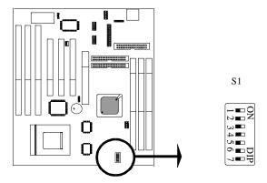
S1 Pin 1 to Pin 3: CPU Ratio Selector
