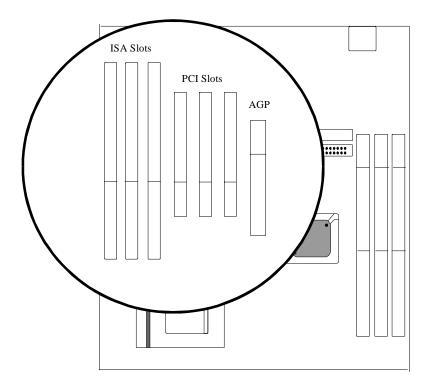
AGP (Accelerated Graphic Port) is the new bus standard that allows the bus speed to run at 66 MHz with up to 133 MHz data transfer capabilities, which is four times as fast as that of the PCI bus. At this speed, the AGP graphic cards can transfer data up to 528MB/second. This high transfer capabilities enables 3D graphic applications, multiple media applications, uncompressed to run smoothly and display in broadcasting quality.
