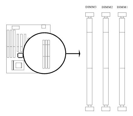
Insert the module as shown. Due to different number of pins on either side of the breaks, the module will only fit in the orientation as shown.
