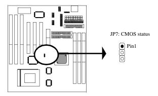
*JP7* is a 3-pin connector. Clear CMOS if system password is forgotten. Below is details to show how to clear CMOS.
