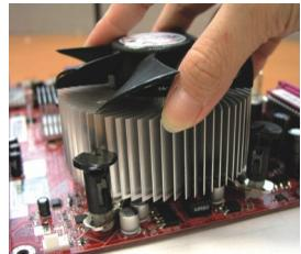
4. Press down the white bar on each clip to fasten the fan set on the retention module.
