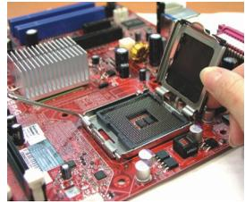
Affix the CPU by pressing the lever downward and locking it beside the socket.
