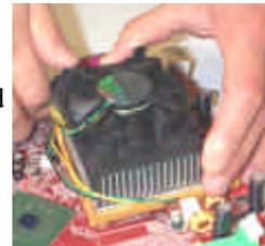
4. Press down the white bar on each clip to fasten the fan set on the retention module.
