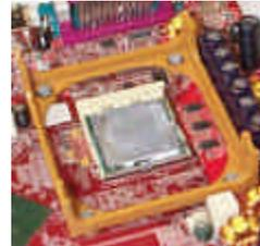
Affix the CPU by pressing the lever downward and locking it beside the socket.
