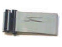
The colored stripe (indicated by the arrow head, right) of the ribbon cable must be the same side with the Pin 1.
