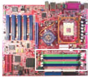
2. Install DDR DIMM straight down into the socket 1 using both hands, then socket 2, and so forth.
