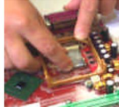
Apply some thermal materials, such as paste or tape, on the CPU top; and install a fan with heatsink that approved by CPU manufacturer to avoid CPU damage. For detail information, please refer to the CPU manufacturer website.
