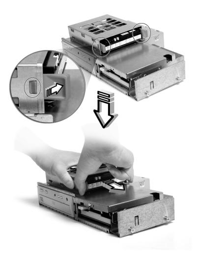
5 Slide the hard disk frame to the left (d); then gently move it out (e) and pull it up to detach it (f).
