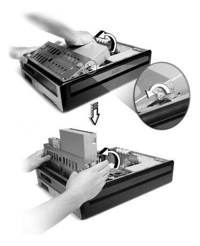
4 Pull out the drive rails that holdthe hard disk to the housing. Set the drive rails aside.
