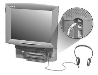
• external speakers: connect to the Audio-out/Line out jack (ime port) located on the left panel of your computer.
