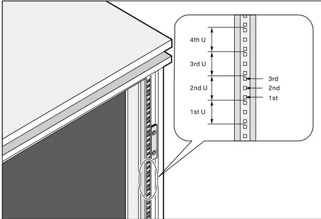
The system occupies 1U in the rack. Count the U positions and hole numbers from the bottom up.
