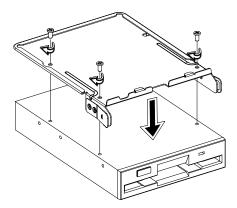
6 Insert the drive carrier with the newly-installed floppy drive into the drive bay.
