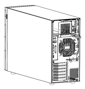
2 Slide the power supply module into the empty bay until you feel resistance.
