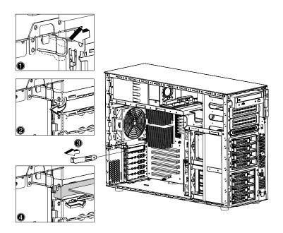
9 Press the PCI slot lock lever on the rear panel of the server.
