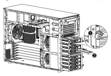
5 Reinstall the air baffle and the chassis panels.
