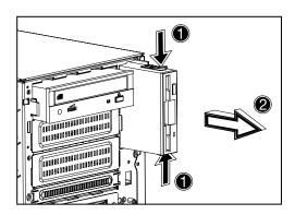
4 Remove the three screws that hold the old drive to the drive carrier then pull it out.
