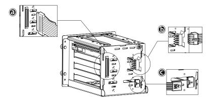
3 Attach the other end of these cables to the corresponding connectors on the mainboard.
