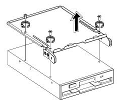
5 Install a new 3.5-inch drive to the drive carrier then secure it with the three screws you have removed earlier.
