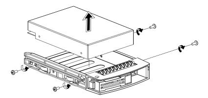
4 Install a hard disk on the hard disk carrier then secure it with the four screws you have removed earlier.
