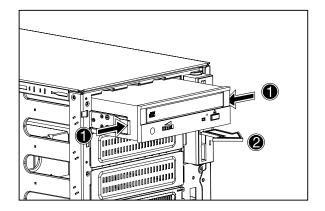
4 Remove the eight screws that hold the old drive to the drive carrier then pull it out.
