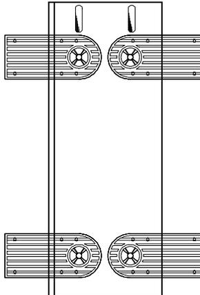
For a standalone system, rotate the legs outward to stabilize the housing.
