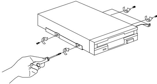
5. Insert the drive into the drive bay and secure it with a screw.
