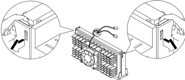
5. Locate the fan connectors on the system board and connect the fan cables.
