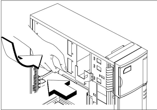
15. Secure the holding plate with the screws that you removed earlier.
