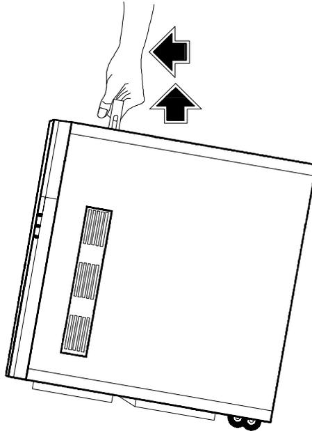
The housing has a handle on top and two wheels behind the feet to facilitate moving to short distances.
