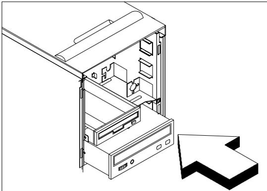
5. Connect the signal and power cables to the drive.
