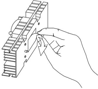
2. Insert the wide clip ends into the wide holes on the processor and the narrow clip ends into the narrow holes.
