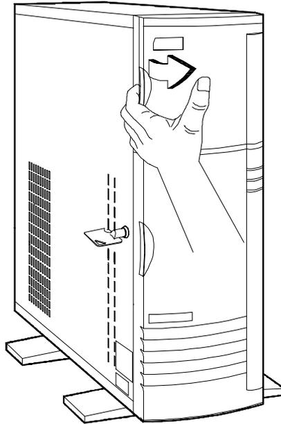
Hold the left edge of the upper front panel to open it and gain access to the diskette drive bays.
