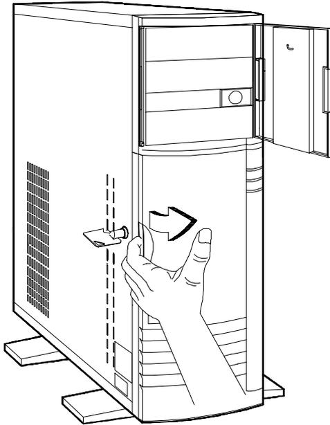
Unlock the housing with the key. Pull the lower panel to access the drive trays.
