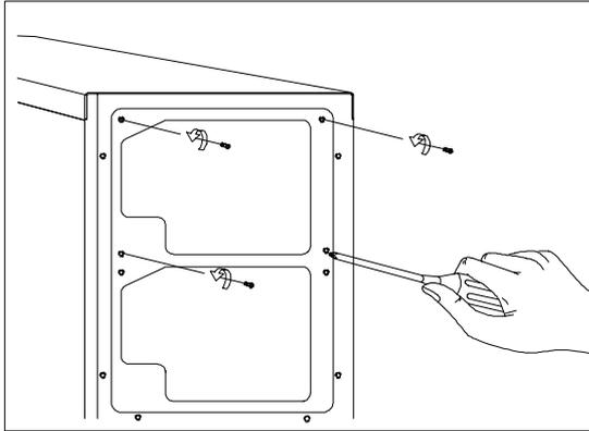
10. Remove the screws that secure the power supply module. In the process, make sure to support the module with your hand.
