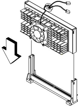
4. Press the latches on the sides to lock the processor module into place.
