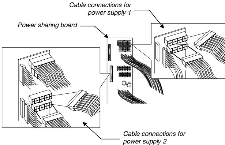
8. Arrange all the cables from the power sharing board and fans to facilitate connection to the system board and disk drives. Do not let power cables block the housing exhaust and fans.
