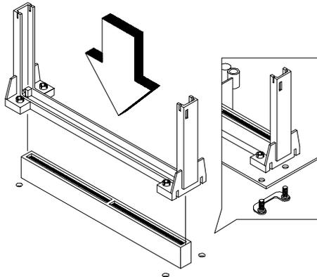
2. With the processor module golden fingers pointing downward, align the processor to the posts of the retention mechanism then lower it down.
