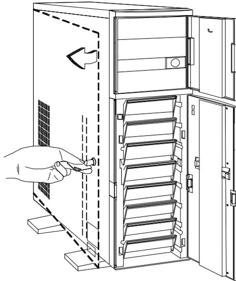
Pull on the key to swing the left panel open. If necessary, you may use a screwdriver to pry open the panel.
