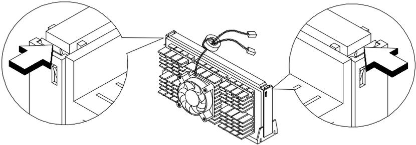
3. Firmly hold the processor module and pull it out of the socket.
