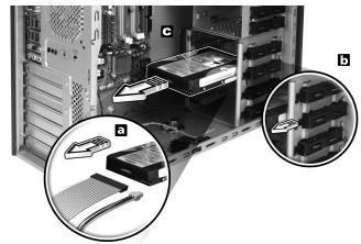
Insert the new hard disk into the frame (a).
