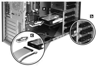
**Note:** Make sure that the other ends of the disk cables are securely connected to their corresponding connectors on the mainboard.
