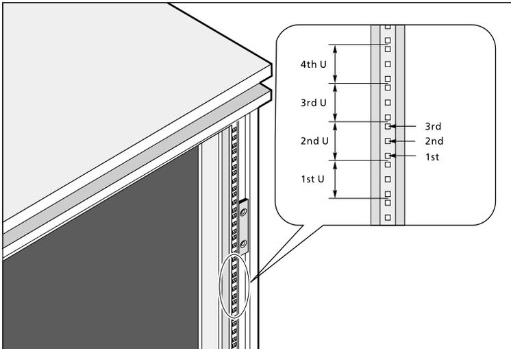
The system occupies 6U in the rack. Count the U positions and hole numbers from the bottom up.
