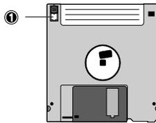
Sliding the write-protect tab to the not-write-protect position (2) will allow you to store and modify data in your diskettes.
