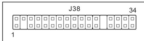
The following below lists the pin-out of the J38 header.
