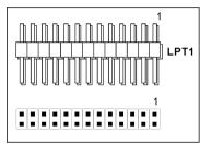
• These headers provide connection to external LPT1 bracket through an extension cable.
