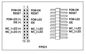
• These headers provide connection to the switches and indicators at font panel.
