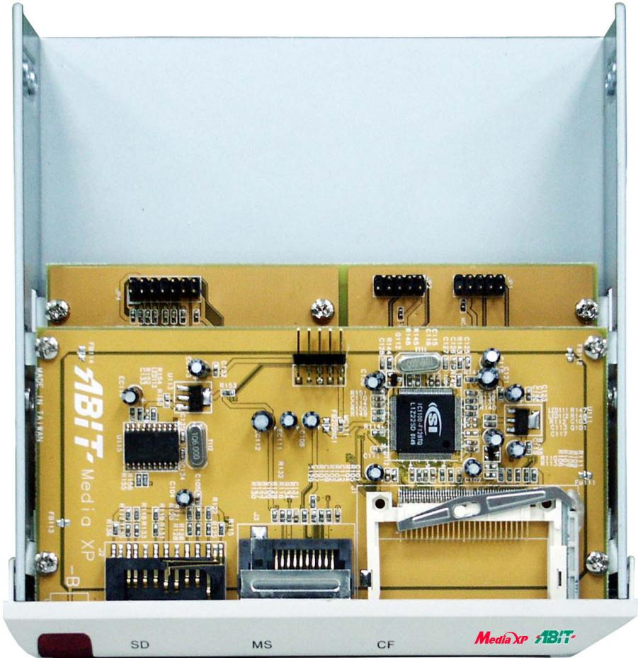
Figure 1-2. Top view of ABIT Media XP/Media XP Pro adapter
