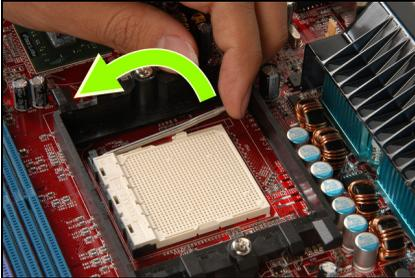
1. Pull out the socket locking lever slightly, then lift it up.
