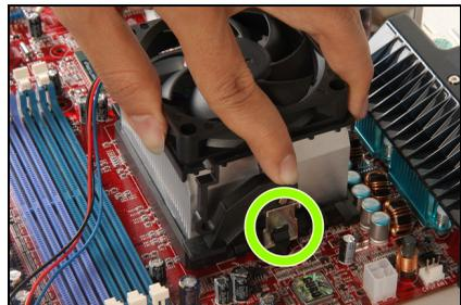
5. Place the heatsink and fan assembly onto the retention frame. Match the heatsink clip with the socket mounting lug. Hook the spring clip to the mounting lug.
