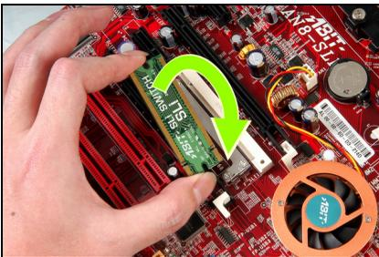
2. Flip the switchboard over to the side labeled with "SLI". Carefully insert the switchboard into the slot.
