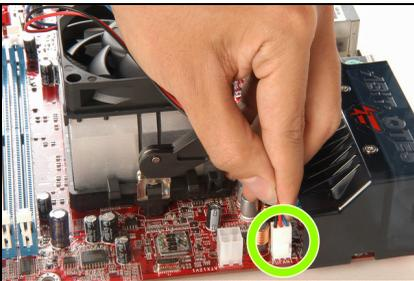
8. Attach the four-pin power plug from the heatsink and fan assembly to the CPU FAN connector.
