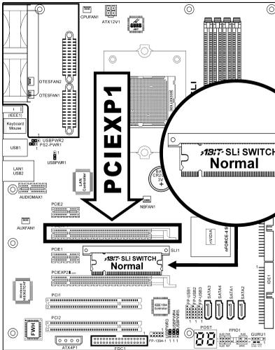
**Normal Mode:** Leave the SLI Switch to its default Normal mode and insert the graphics card into PCIEXP1 slot. The PCIEXP2 slot functions as a PCIE x1 slot under this mode.
