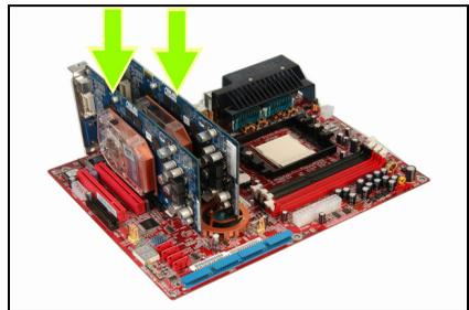
4. Insert the two graphics cards into PCIEXP1 and PCIEXP2 slots on the motherboard.
