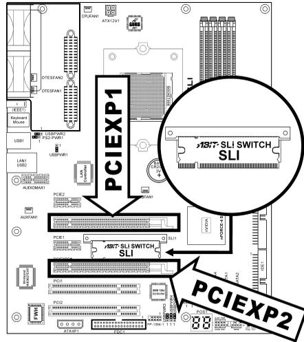
**SLI Mode:** Switch the SLI Switch to SLI Mode and insert the SLI-ready graphics cards into PCIEXP1 and PCIEXP2 slots.
