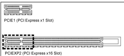
**NOTE:** When PCIEXP2 slot functions as a PCIE x1 slot under **Normal mode**, insert the PCIE x1 card into the marked area of PCIEXP2 slot.
