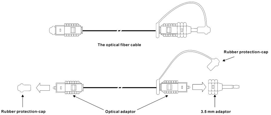
**Note:** Remove the rubber protection-caps before using this optical fiber cable.
