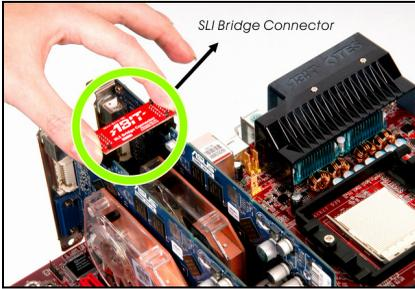
6. Insert the SLI Bridge Connector into the SLI goldfingers on each graphics card.
