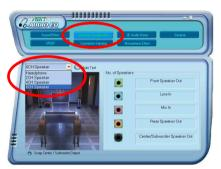
**4.** In this "Speaker Configuration" tab, select [6CH Speaker] to enable 6-channel audio system
