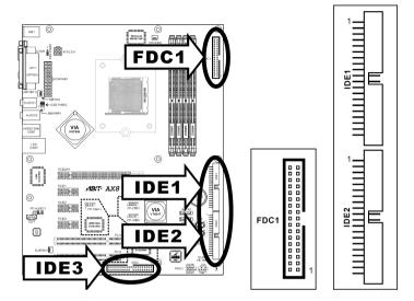
The FDC1 connector connects up to two floppy drives with a 34-wire, 2-connector floppy cable. Connect the single end at the longer length of ribbon cable to the FDC1 on the board, the two connectors on the other end to the floppy disk drives connector. Generally you need only one floppy disk drive in your system.
