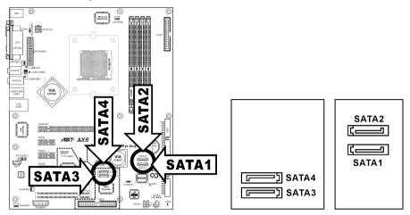
NOTE: The connectors [SATA1] and [SATA2] provide "RAID 0" or "RAID 1" service besides their regular SATA connection. For models "AX8-3<sup>rd</sup> Eye" and "AX8", additional "RAID 0+1" and "JBOD" services are provided further.
