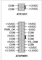
**NOTE:** It is recommended to connect to a power supply with 350W, 20A +5VDC capacity at least for heavily loaded system, and a 2A +5VSB capacity at least for supporting wake-up features.
