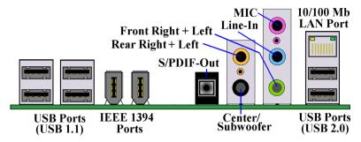
Figure 2-9. AT7 back panel connectors
