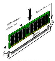
Figure 2-6. DDR DIMM module installation
