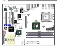
FPIO1 are for switches and indicators for the chassis's front panel, there are several functions that come from this header. You have to watch the pin position and the orientation, or you may cause LED do not light up. Figure below shows you the FPIO1 functions of the pins.
