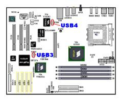
Thess headers are for connecting the additional USB port plugs. Each connector can provides two additional USB plugs. Which means, total you can get two additional USB plugs from each connector. You can use the special USB port expansion cable to connect it (the cable come with the metal plate can fixed on the back panel of computer chassis).
