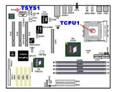
The TCPU1 is used to detect the CPU temperature. The TSYS1 is used to detect the system environment temperature. You can see the readings in the BIOS or in the hardware monitoring application main screen.
