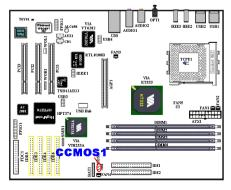
Jumper CCMOS1 used to discharge CMOS memory. When you install the motherboard, make sure this jumper is set for normal operation (pin 1 and 2 shorted). See figure below.
