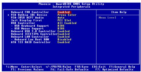
Figure 3-6A. Integrated Peripherals Menu Default Screen
