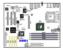
This header is reserved for the system management bus (SM-Bus). The SM-Bus is a specific implementation of an 1<sup>2</sup>C bus. 1<sup>2</sup>C is a multi-master bus, this means that multiple chips can be connected to the same bus and each one can act as a master by initiating a data transfer. If more than one master simultaneously tries to control the bus, an arbitration procedure decides which master gets priority. You can connect the devices which utilizes the SM-Bus.
