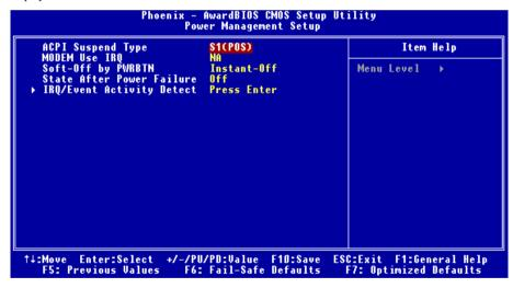
Figure 3-7A. Power Management Setup Main Menu
