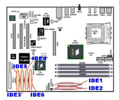
If you want to connect two hard drives together through one IDE channel, you must configure the second drive to Slave mode after the first Master drive. Please refer to the HDD documentation for jumper settings. The first drive connected to IDE1 is usually referred to as "Primary Master", and the second drive as "Primary Slave". The first drive connected to IDE2 is referred to as "Secondary Master" and the second drive as "Secondary Slave".
