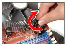
**11.** Rotate the fastener clock-wise to lock the heatsink and fan assembly into position.
