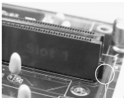
Figure 13 - Pentium II Slot Connector and Key Pin
