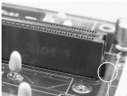
Pentium II Slot Connector and Key Pin
