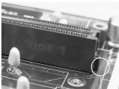
Figure 14 Pentium II Slot Connector and Key Pin
