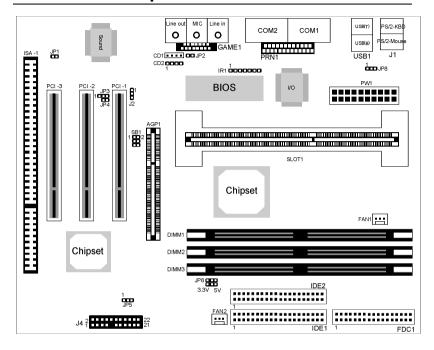
Figure 2-1. Mainboard Component locations
