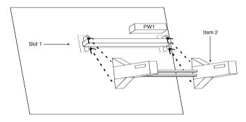
If the retention clip is installed incorrectly, you will not be able to insert the retention clip into the CPU and in this situation you might need to rotate the retention clip by  $180^{\circ}$ .
