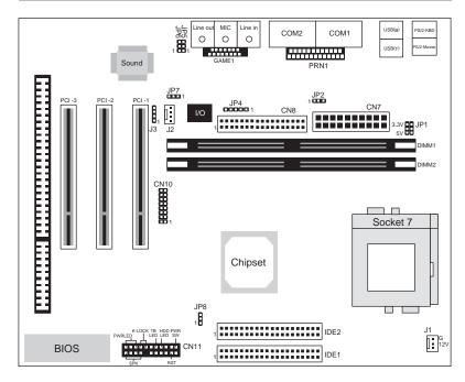
Figure 2-1. Mainboard Component locations
