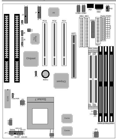
Figure 2–1. Mainboard Component Locations
