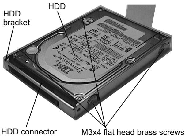
5. Remove **four M3x4 brass flat head screws** securing the HDD to the bracket and lift the drive out of the **bracket**.
