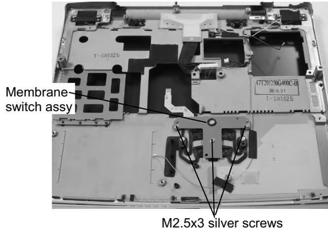
1. Remove **three M2.5x3 flat head silver screws** securing the membrane switch.
