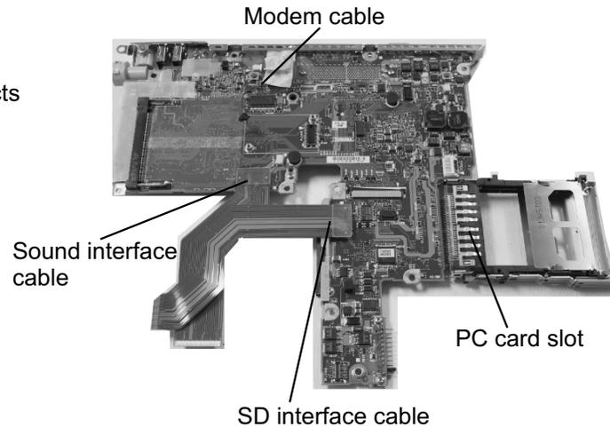
4. Remove the **PC card slot** from PJ117 on the top PCB.
