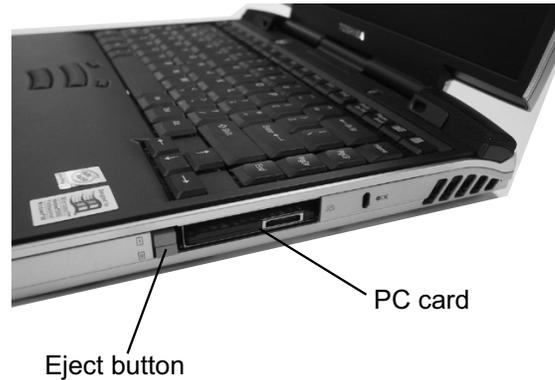
1. Press the **eject button** for the PC card you want to remove.
