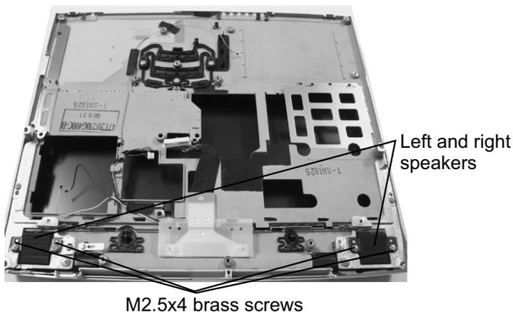
1. Remove **four M2.5x4 brass screws** securing the left and right speakers.
