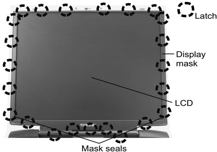
1. Remove **two mask seals** at the bottom corners of the display assembly using a pair of fine-tipped tweezers.
