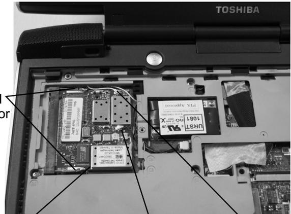
Mini-PCI connector clips
