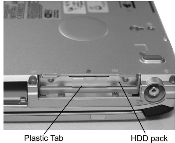
4. Unfold the **plastic tab** and pull to remove the HDD from the bay.
