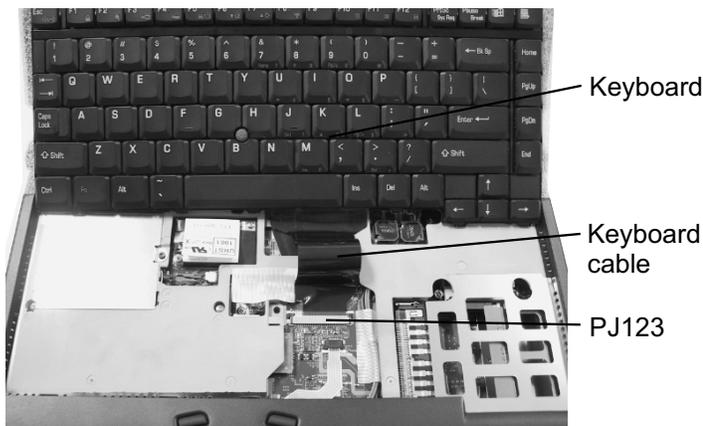
5. Lift out the **keyboard** and set it as shown above (Place an insulator between the keyboard and the LCD to prevent scratches on the LCD).
