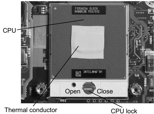
1. Peel off the **thermal conductor**.
