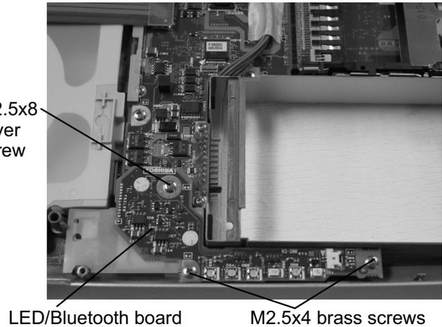
1. Remove **two M2.5x4 brass screws** and **one M2.5x8 silver screw** securing the LED/Bluetooth board.
