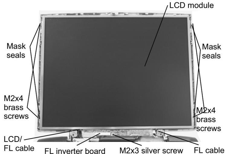
1. Remove **one M2x2.8 silver screw** securing the FL inverter board.
