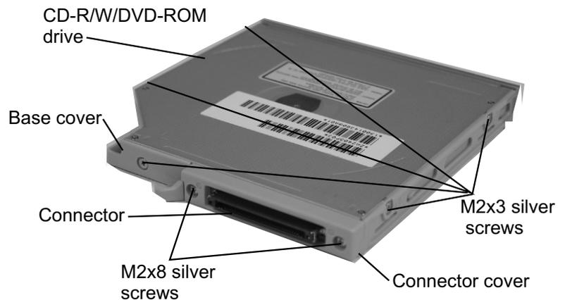
1. Remove **five M2x3 silver screws** securing the base cover and lift off the **base cover**.
