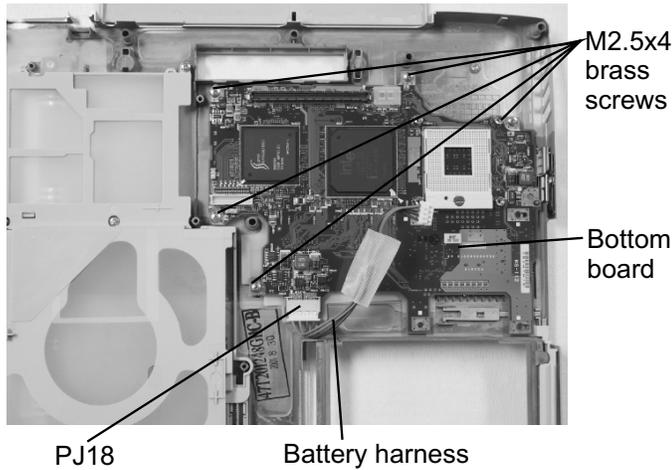
1. Disconnect the **battery harness** from **PJ18** on the bottom PCB.
