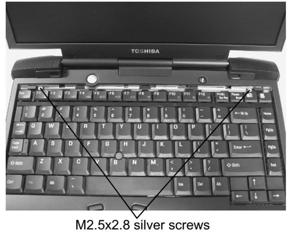
2. Turn the computer right side up and open the display panel.
