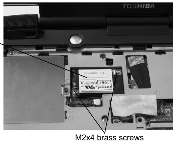
1. Remove **two M2x4 brass screws** securing the modem board.
