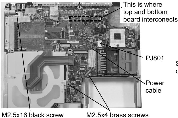
1. Disconnect the **power cable** from **PJ801** on the top PCB.
