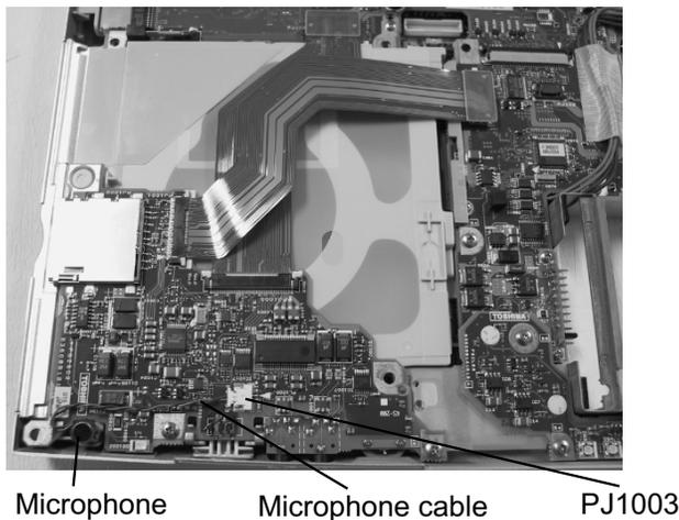
1. Disconnect the **microphone cable** from **PJ1003** on the SD/Sound board.
