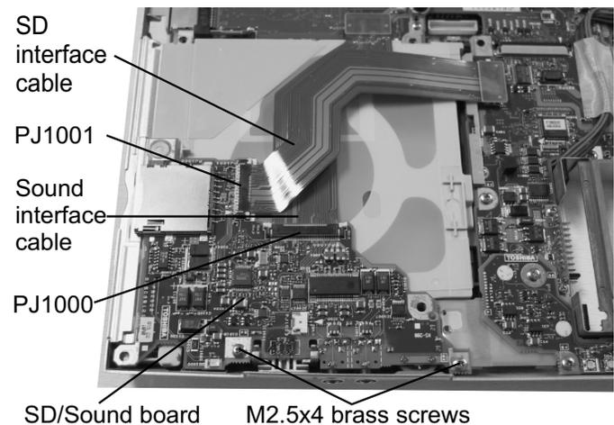
1. Disconnect the **SD interface cable** from **PJ1001** and **sound interface cable** from **PJ1000** on the **SD/sound board**.
