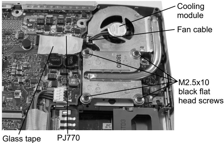
1. Remove the **glass tape** securing the fan cable and disconnect the **cable** from **PJ770** on the top board.
