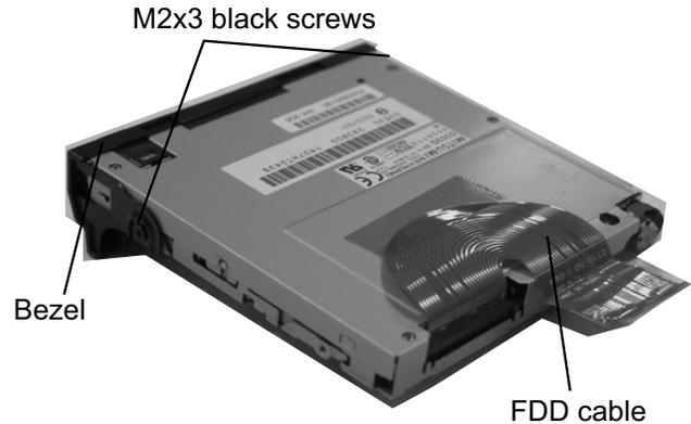
1. Remove **one M2.5x4 black screw** securing the FDD assembly.
