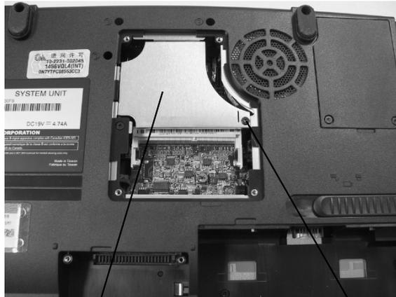
Mini PCI slot cover      M2.5x4 black torx screws
